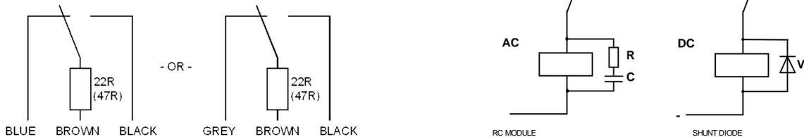
Overloading of the magnetic switch can result in damage to the built-in reed contact. This can lead to a malfunction of the downstream control and to physical injury or property damage. You **MUST** ensure that the switch rating maximum values given in the technical data are adhered too.
